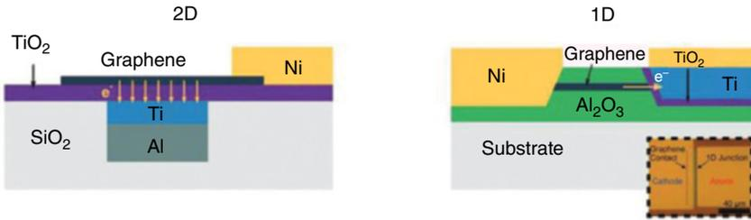
**Figure 1.10** Schematic of the 2D (left) and 1D (right) MIG diodes. Source: Wang et al. [49]/ John Wiley & Sons.
