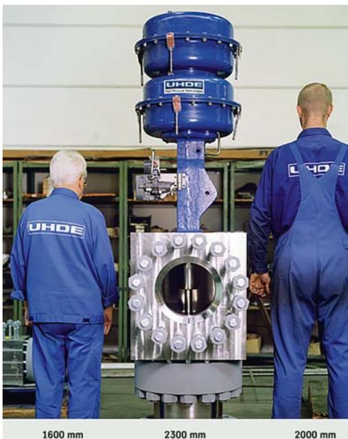
Control valve of a urea plant. Source: Courtesy of Uhde, Germany.
