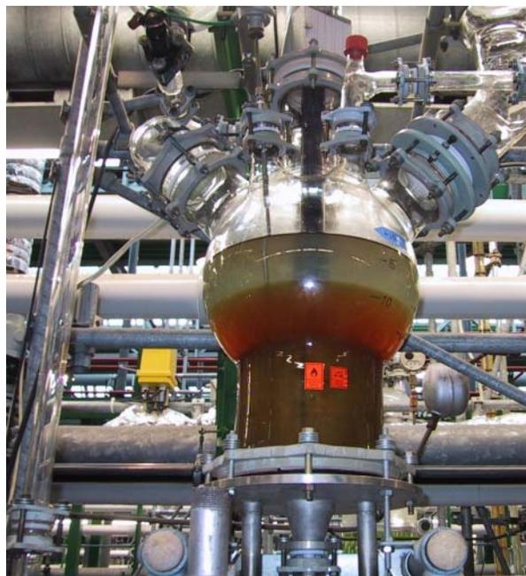
Photograph of a homogeneously catalyzed, liquid-liquid biphasic reaction.
