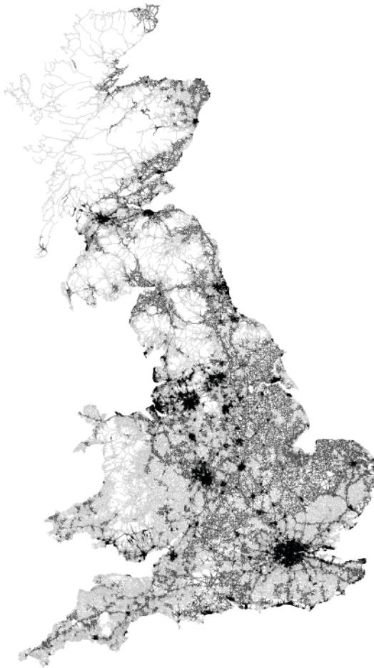
Figure 1.3 Differences in road morphology are clearly distinguished by a neural network, here revealing natural clusters which correspond with actual land use designations. (Source: redrawn from Varoudis and Penn 2020).
