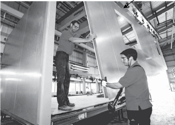
Photograph 2.2 Factory production of a timber-framed house. Insulation and windows installed (a); exterior timber cladding being fixed (b).
