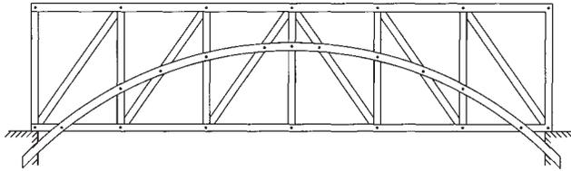
**Fig. 1.3** Arched truss—designed by Theodore Burr, patented 1817. (From *Bridges and Men* by Joseph Gies. Copyright © 1963 by Joseph Gies. Used by permission of Doubleday, a division of Bantam Doubleday Dell Publishing Group, Inc.)
