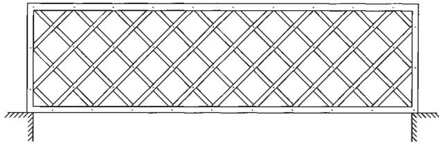
**Fig. 1.5** Lattice truss—designed by Ithiel Town, patented 1820. (From *Bridges and Men* by Joseph Gies. Copyright © 1963 by Joseph Gies. Used by permission of Doubleday, a division of Bantam Doubleday Dell Publishing Group, Inc.)
