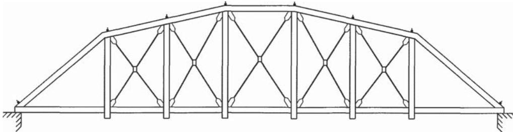
**Fig. 1.9** Bowstring arch—designed by Squire Whipple, patented in 1841.
