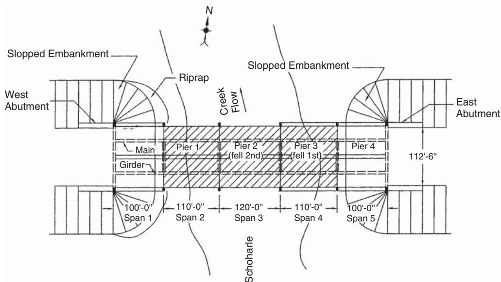
Fig. 2.9 Schematic plan of Schoharie Creek Bridge. (NTSB, 1988).
