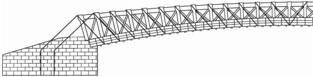
**Fig. 1.2** Trussed arch—designed by Lewis Wernwag, patented 1812.
