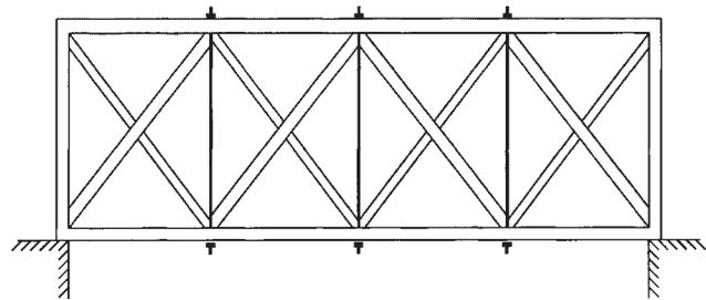
**Fig. 1.7** Howe truss—designed by William Howe, patented in 1841. (From *Bridges and Men* by Joseph Gies. Copyright © 1963 by Joseph Gies. Used by permission of Doubleday, a division of Bantam Doubleday Dell Publishing Group, Inc.)
