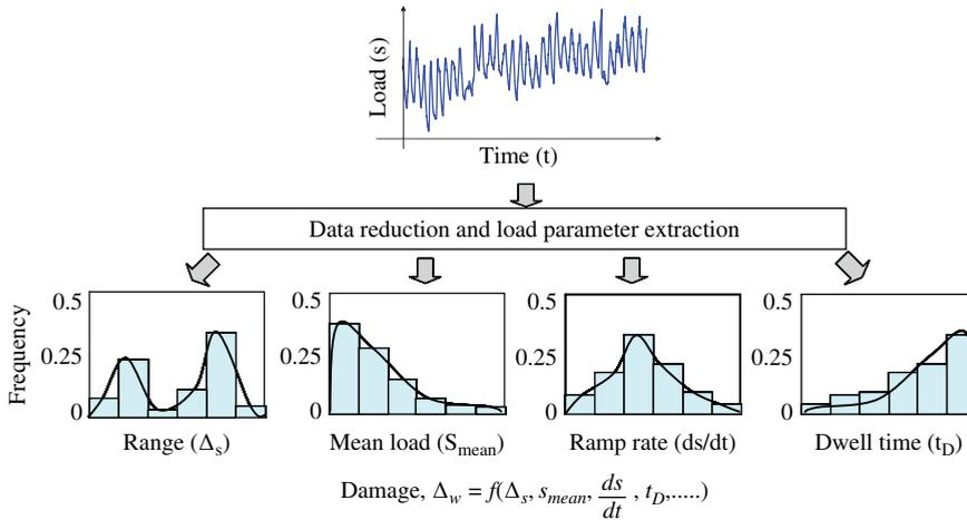
Figure 1.7 Load feature extraction.
