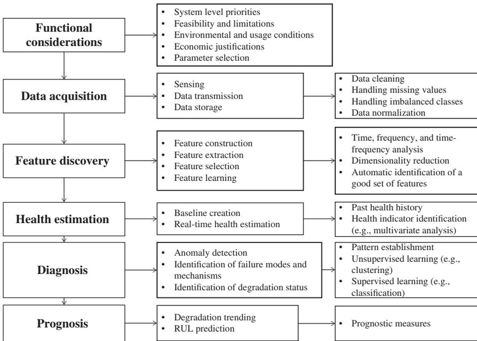
Figure 1.10 A general procedure of a data-driven approach to prognostics.
