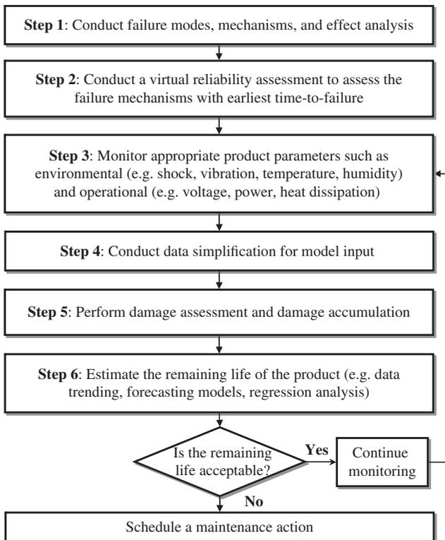
**Figure 1.5** CALCE life consumption monitoring methodology.
