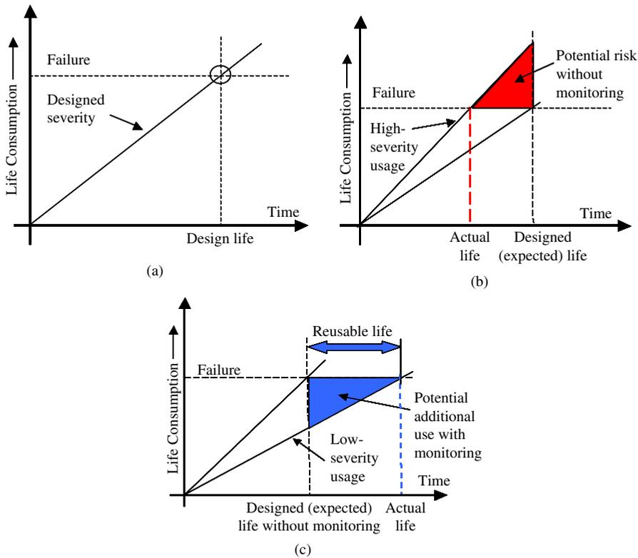
**Figure 1.2** Application of health monitoring for product re-use. (a) Usage as per design, (b) More severe usage than intended design, and (c) Less severe usage than intended design.
