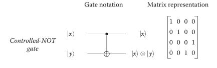
The schematic representation of the CNOT gate is given here. The truth table of this gate is presented below.
