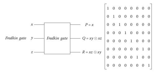
The gate notation and matrix representation of the Fredkin gate are presented here. The truth table of this gate is shown below.
