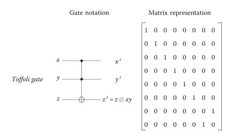
The gate notation and matrix representation of the Toffoli gate are presented here. The truth table of this gate is given below.
