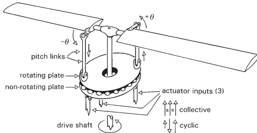
Fig. 2.5 Rotor control through a swash plate
