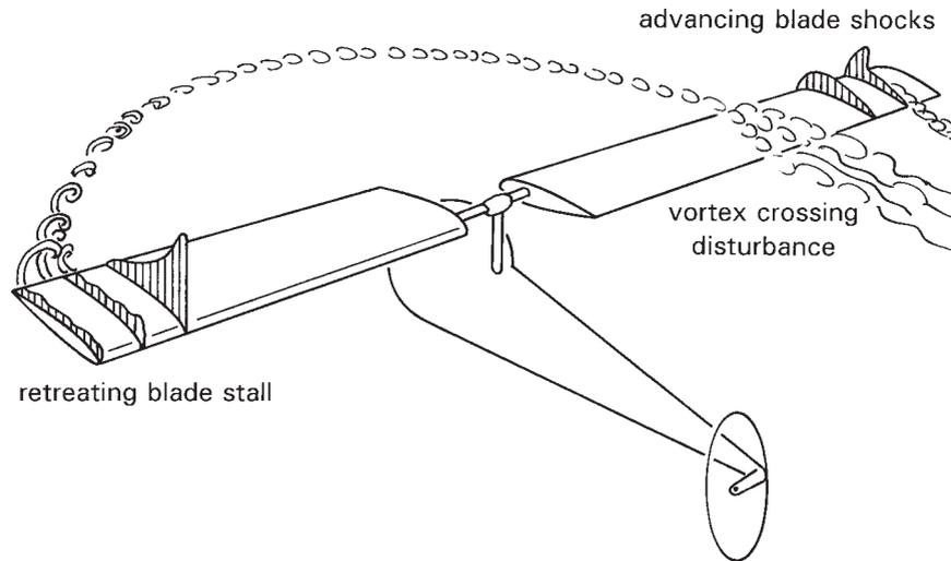
**Fig. 2.9** Features limiting rotor performance in high-speed flight
