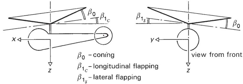
**Fig. 2.20** The three rotor disc degrees of freedom
