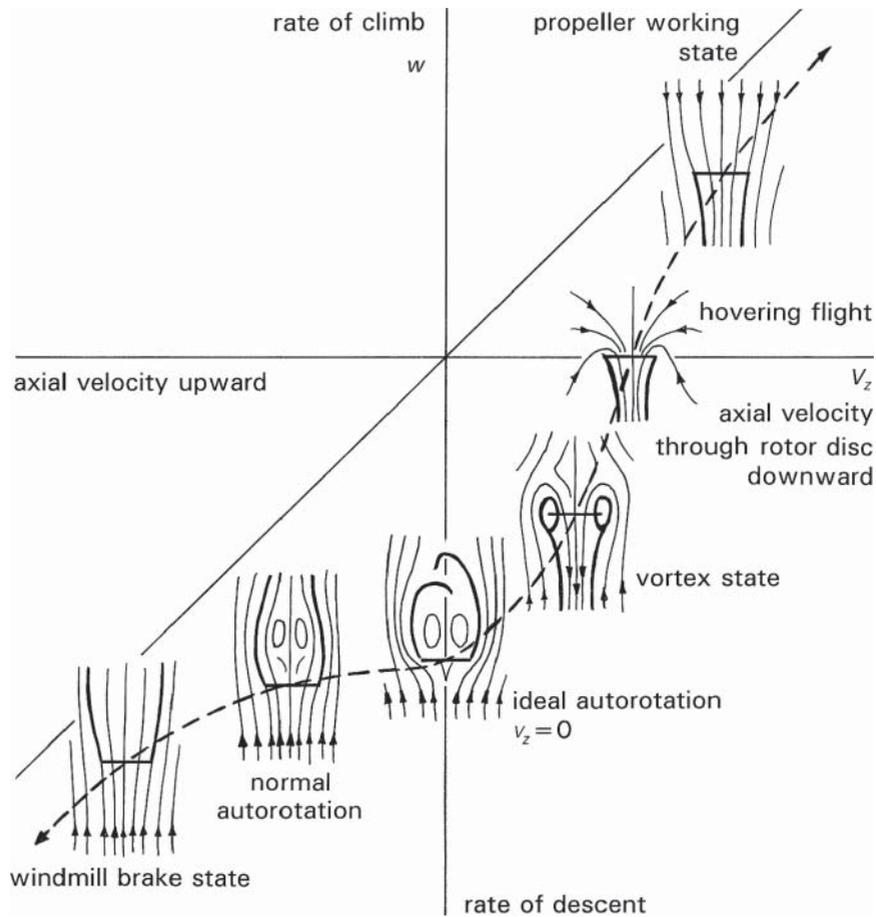
Fig. 2.8 Rotor flow states in axial flight
