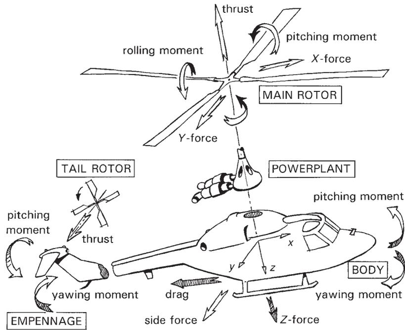
Fig. 2.15 The modelling components of a helicopter
