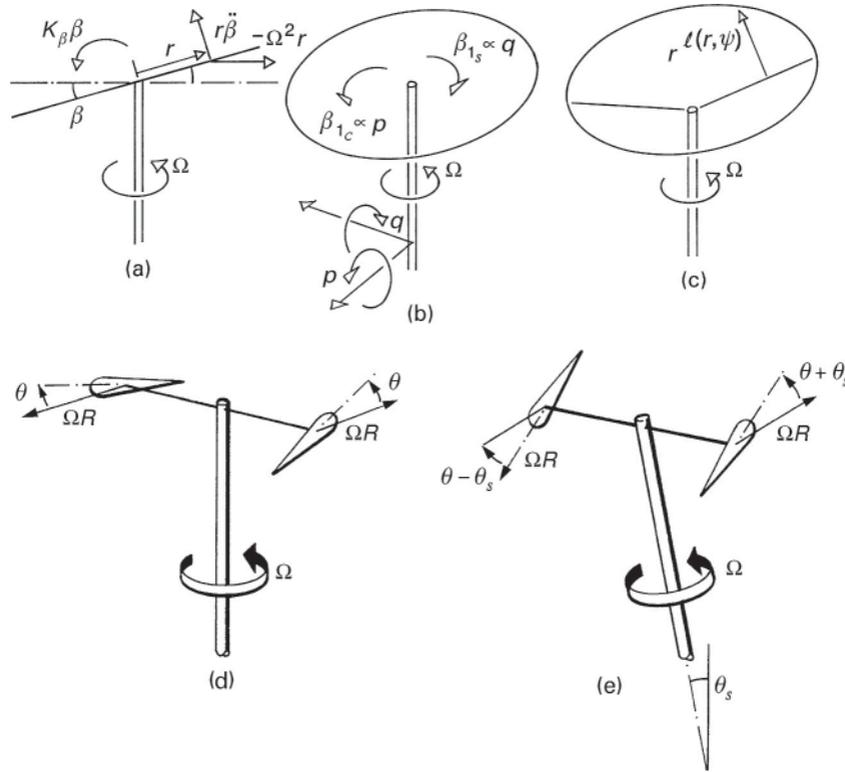
**Fig. 2.18** Sketches of rotor flapping and pitch: (a) rotor flapping in vacuum; (b) gyroscopic moments in vacuum; (c) rotor coning in air; (d) before shaft tilt; (e) after shaft tilt showing effective cyclic path
