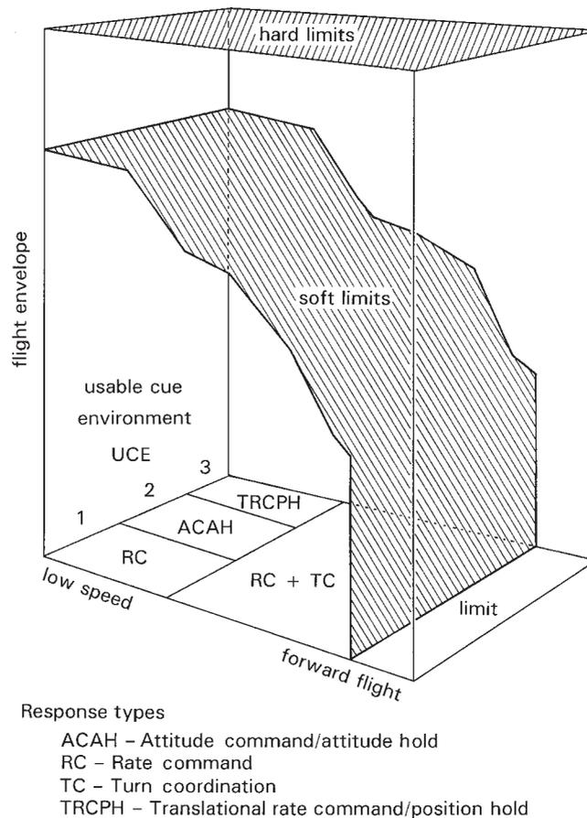
**Fig. 2.13** Response types required to achieve Level 1 handling qualities in different UCEs
