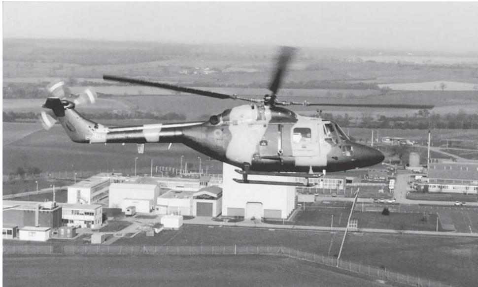
*The DRA research Lynx ALYCAT (Aeromechanics LYnx Control and Agility Testbed) shown flying by the large motion system of the DRA advanced flight simulator (Photograph courtesy of Simon Pighills)*
