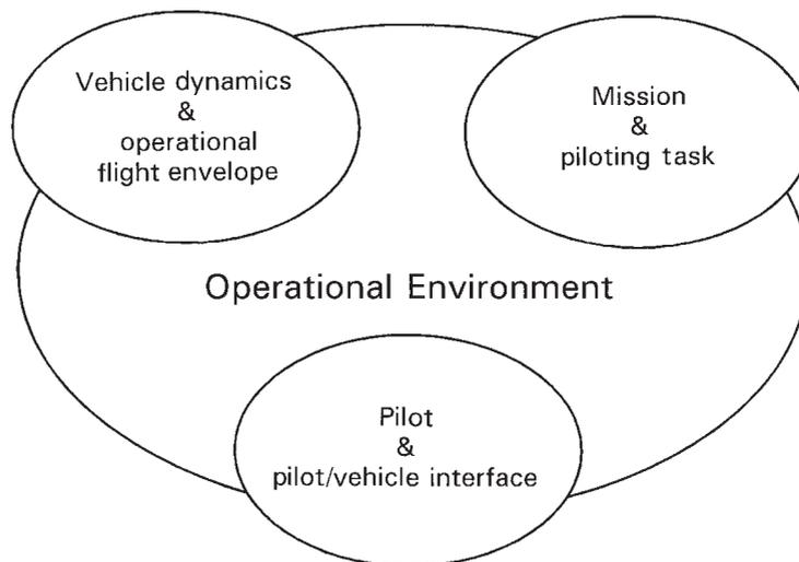
**Fig. 2.1** The four reference points of rotorcraft flight dynamics
