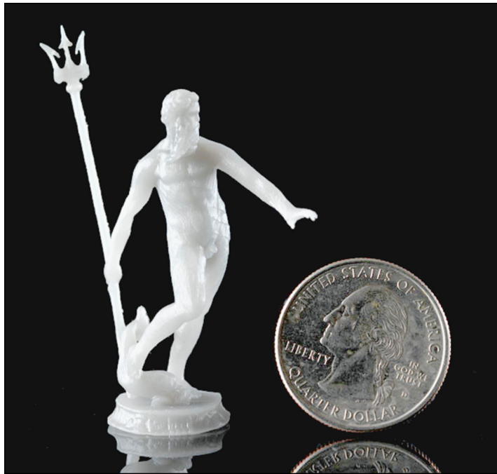
FIGURE 2-3: Object created via stereolithography on a FormOne printer.
