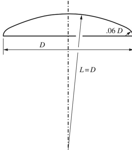
**Figure 1.13** Elliptical head with  $a/b = 2.96$  ratio
