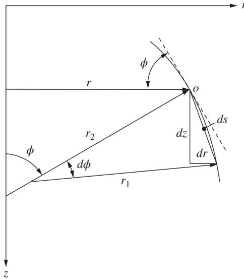
**Figure 1.3** Shell geometry
