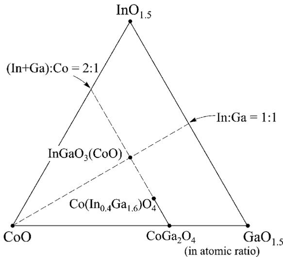
**Figure 1.6** Phase equilibrium diagram in the  $\text{In}_2\text{O}_3\text{--Ga}_2\text{O}_3\text{--CoO}$  system at  $1300^\circ\text{C}$ . Plotted are  $\text{YbFe}_2\text{O}_4$ -type  $\text{InGaO}_3(\text{CoO})$  and spinel-type  $\text{CoGa}_2\text{O}_4$ . Indium solid solution of  $\text{CoGa}_2\text{O}_4$  exists up to  $\text{In}_{0.4}\text{Ga}_{1.6}\text{O}_3(\text{CoO})$ . The solid line shows the indium solid-solution range of  $\text{CoGa}_2\text{O}_4$ . Source: Adapted from [9]
