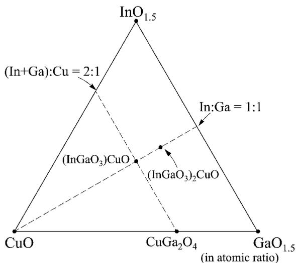
**Figure 1.5** Phase equilibrium diagram in the  $\text{In}_2\text{O}_3\text{-Ga}_2\text{O}_3\text{-CuO}$  system at  $1000^\circ\text{C}$ . ● Indicates that  $\text{InGaO}_3(\text{CuO})$  and  $(\text{InGaO}_3)_2\text{CuO}$  are isostructural with  $\text{YbFeO}_3(\text{FeO})$  and  $(\text{YbFeO}_3)_2\text{FeO}$ , respectively. *Source:* Adapted from [9]
