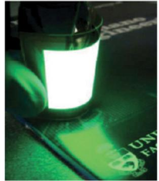
**FIGURE 2.5** (a) Schematic of the OLED device structure on low-cost flexible plastic with metal electrodes. (b) Photograph of a large-area flexible OLED ( $50 \times 50 \text{ mm}^2$ ) working at high luminance ( $>5000 \text{ cd/m}^2$ ). [Source: Wang *et al.* [48], Figure 1, p. 754. Adapted with permission from Nature Publishing Group.]
