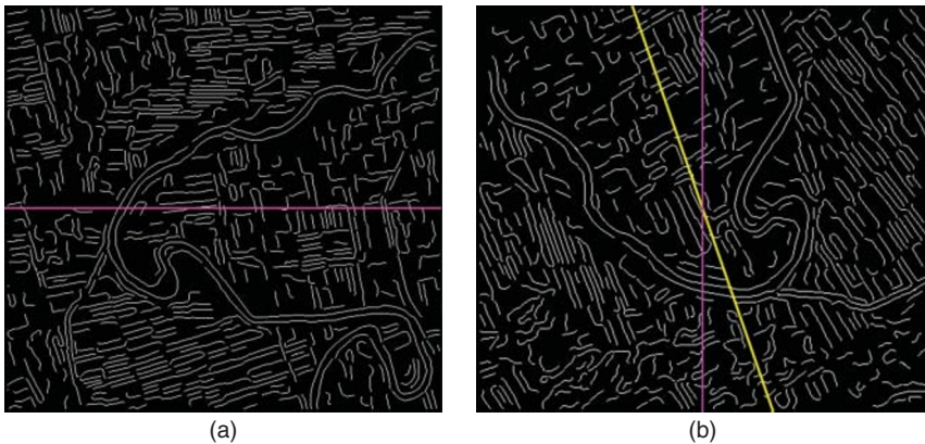
Figure 2.20 (a and b) Canny edges of the radar images (a) and (b) in Fig. 2.14. The orientations detected by geometric gradients and intensity gradients are shown with yellow and purple lines, respectively. The yellow line in (a) is hidden by the purple line and, thus, is not visible.
