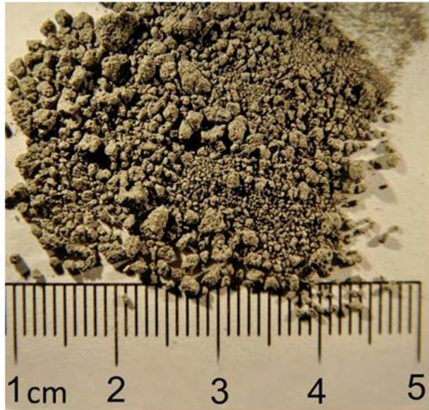
Figure 2. Typical Ungraded Silt Sand (Stockpiled FA 1:3 cement/silt ratio)
