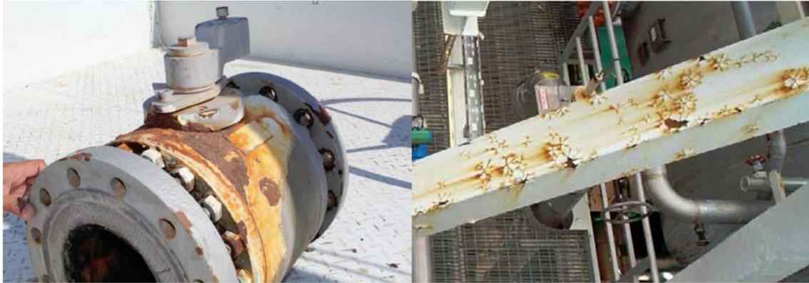
Figure 3. Damaged coating followed by corrosion of the carbon steel substrate material.
