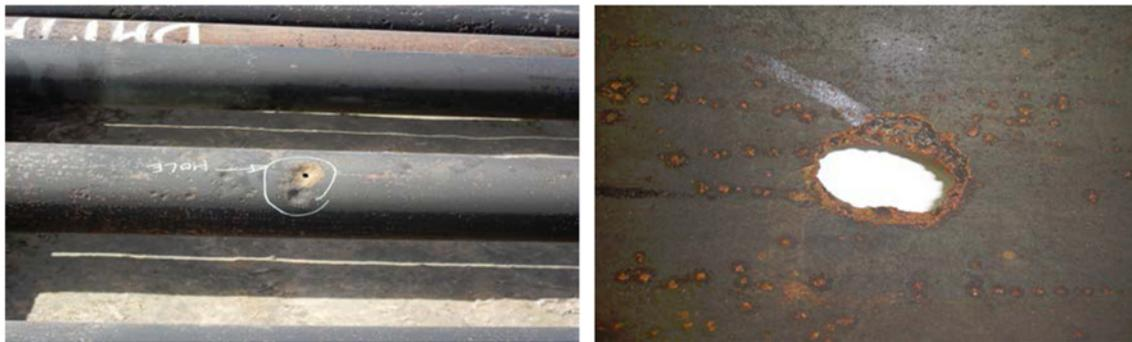
Figure 5. Tubing corrosion – Left: External corrosion including a penetration (hole). Right: The hole seen from the inside of the tubing.
