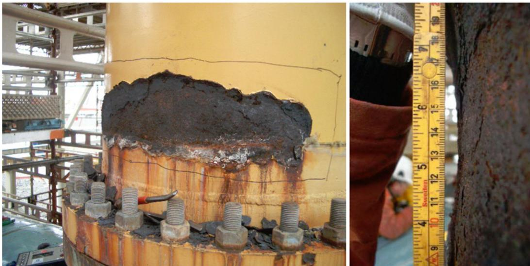
Figure 4. Corrosion under insulation in a storage vessel made from carbon steel.
