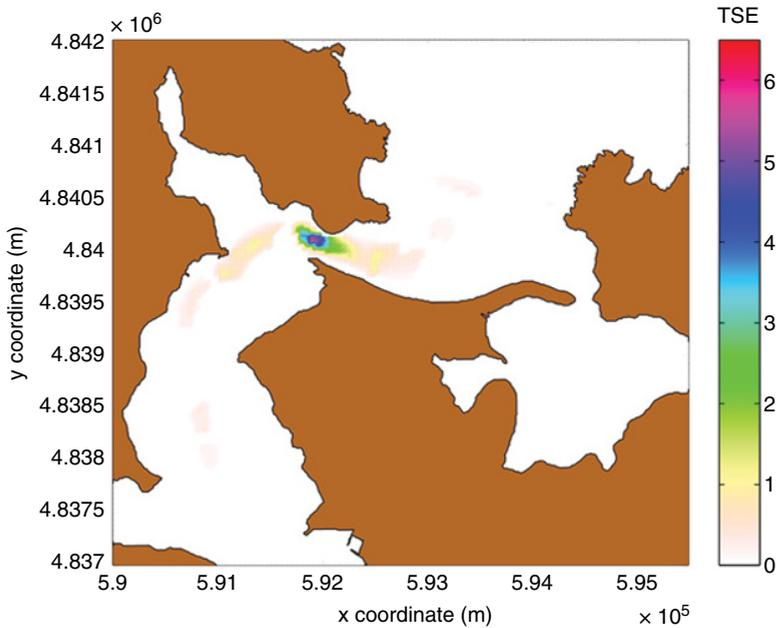
**Figure 2.14** TSE index in the inner estuary. The area with greatest potential for tidal stream exploitation between Pt. Postiña and Pt. Cabalar (Figure 2.13) is conspicuous in the graph.
