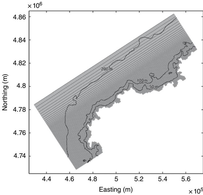
**Figure 2.4** Computational grid for the Death Coast case study. For the sake of clarity, only one in three nodes is represented.
