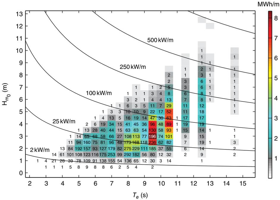
**Figure 2.3** Offshore resource characterisation matrix for the Death Coast (NW Spain), with improved resolution:  $0.5\text{ s } (\Delta T_e) \times 0.5\text{ m } (\Delta H_s)$ .
