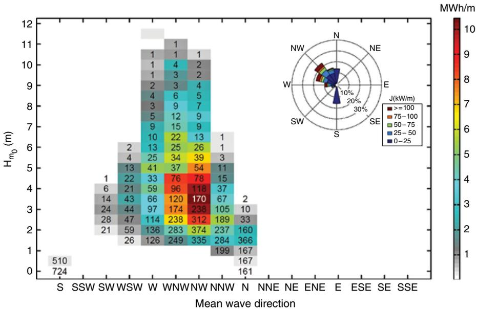
Figure 2.7 Resource characterisation matrix at the nearshore hotspot in terms of mean wave direction and significant wave height ( $\theta_m, H_s$ ). A wave power rose is also included.
