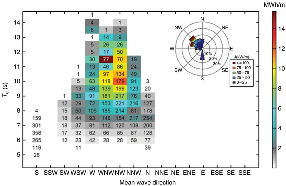
**Figure 2.8** Resource characterisation matrix at the nearshore hotspot in terms of mean wave direction and energy period ( $\theta_m$ ,  $T_e$ ). A wave power rose is also included.
