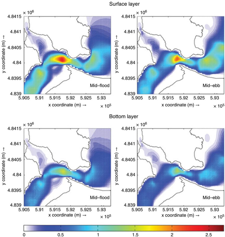
**Figure 2.15** Flow velocity at mid-flood and mid-ebb in the surface and bottom layers of the inner estuary, Ria de Ortigueira (NW Spain).
