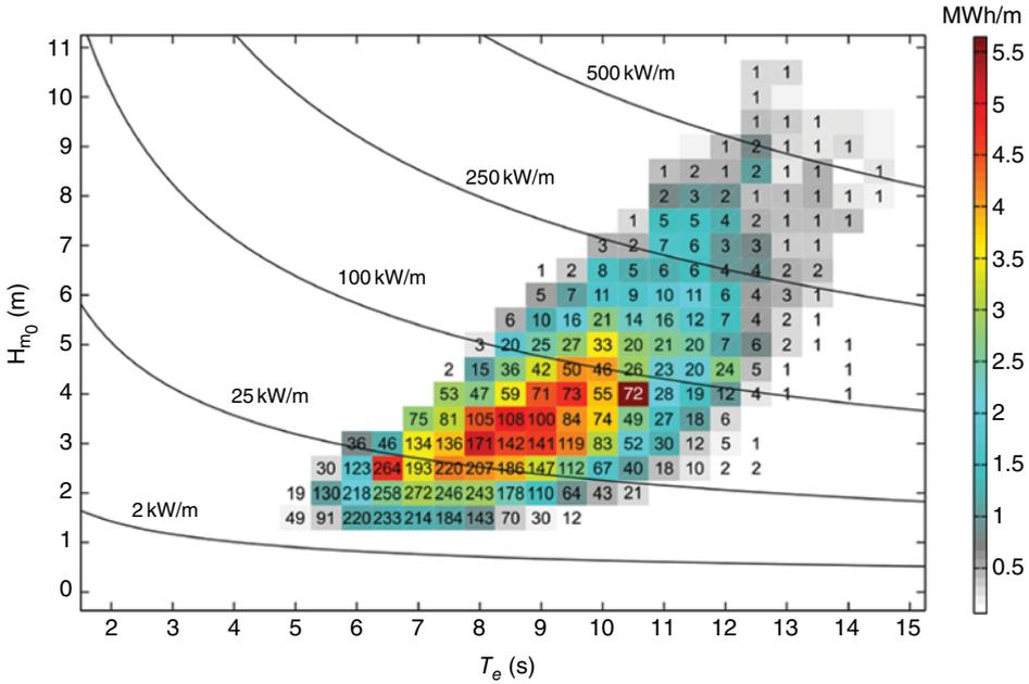
**Figure 2.5** Offshore resource characterisation matrix limited to the wave cases selected for propagation, i.e. 95% of the total resource.
