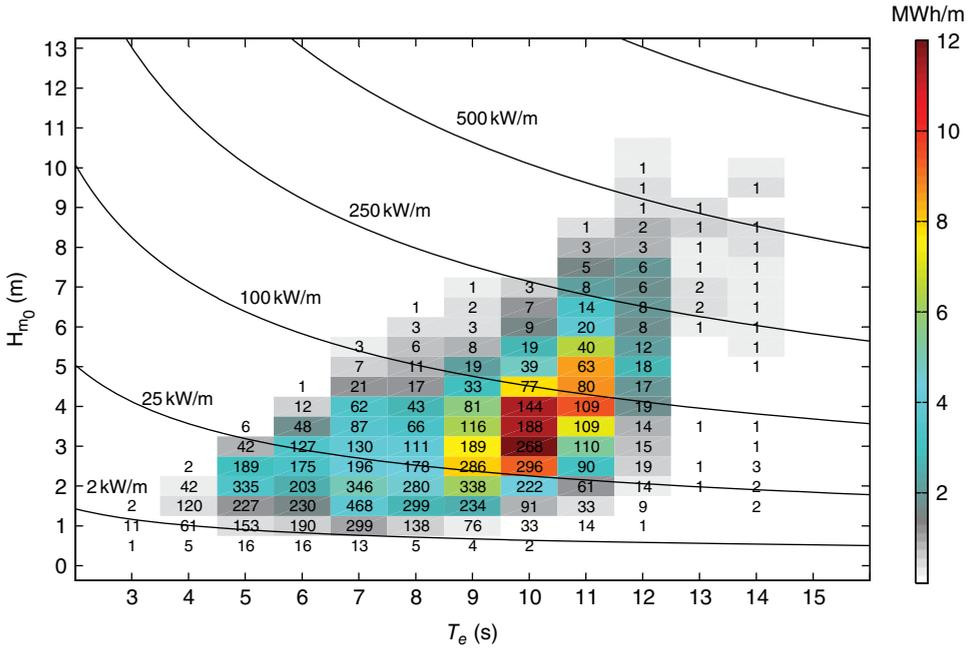
**Figure 2.2** Offshore resource characterisation matrix including wave power isolines for the Death Coast (*Costa da Morte*), Galicia, NW Spain. The numbers in the greyed squares represent the occurrence of the respective energy bins, expressed in hours in a typical year. The greyscale indicates the contribution of each energy bin to the annual resource.
