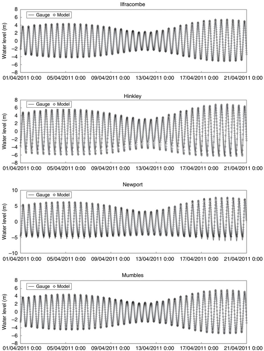
**Figure 2.10** Model validation: observed (gauge) and computed (model) time series of tidal levels at four stations in the Bristol Channel.
