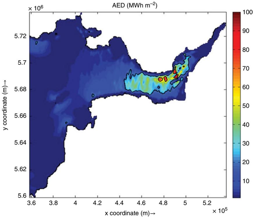
**Figure 2.11** Annual tidal stream energy density ( $\text{MWh m}^{-2}$ ) in the Severn Estuary and Bristol Channel (UK).
