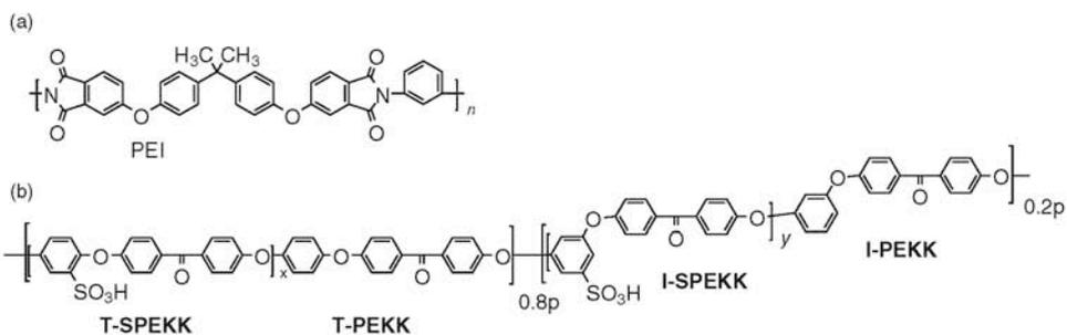
**FIG. 1.7** (a) Poly(ether imide). (b) Sulfonated T-(PEKK-co-PEKK)-co-I-(PEKK-co-PEKK).
