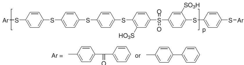
**FIG. 1.3** 3,3'-Sulfonated poly(arylenethioether sulfone) (sPTES).
