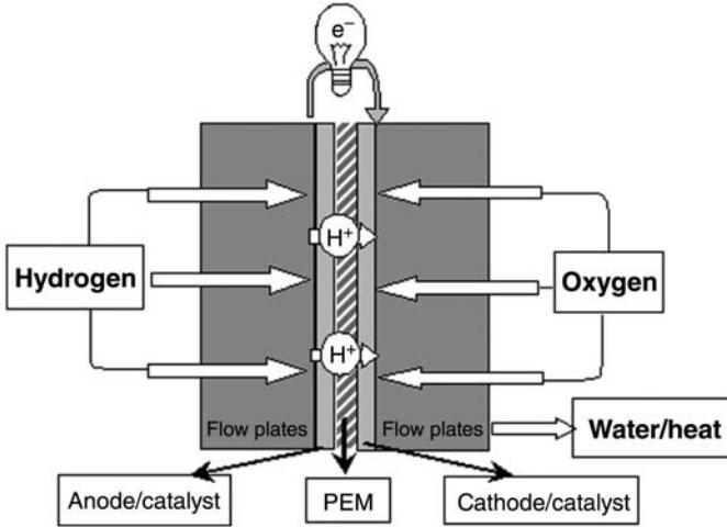
**FIG. 1.1** Schematic drawing of a hydrogen/oxygen fuel cell and its reactions based on polymer electrolyte membrane fuel cell (PEMFC).
