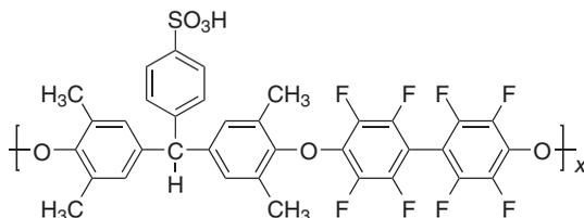
**FIG. 1.5** Poly(fluorinated-arylene ether) with sulfonated triphenyl methane moiety [135,136].
