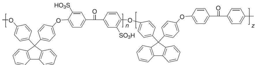
FIG. 1.4 Sulfonated poly(flourenyl ether ketone) (sPFEEK).
