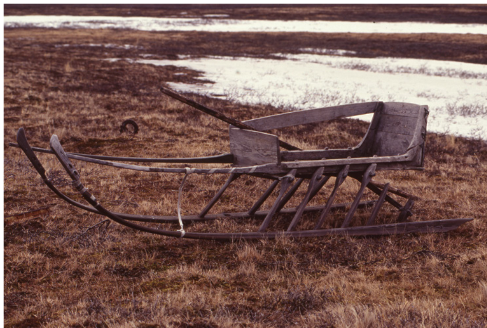
Figure 1.12 Reindeer sledge made only of wood. Western Yamal Peninsula. Source: Photo: Kjell Danell.
