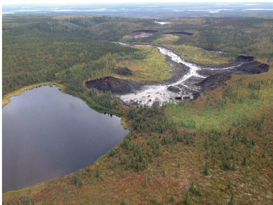
Figure 2.1 A large retrogressive thaw slump on the Peel Plateau near the border between the Yukon and Northwest Territories, Canada. The lake in the bottom left is approximately 140m across. Source: Photo: Michael Pisaric.
