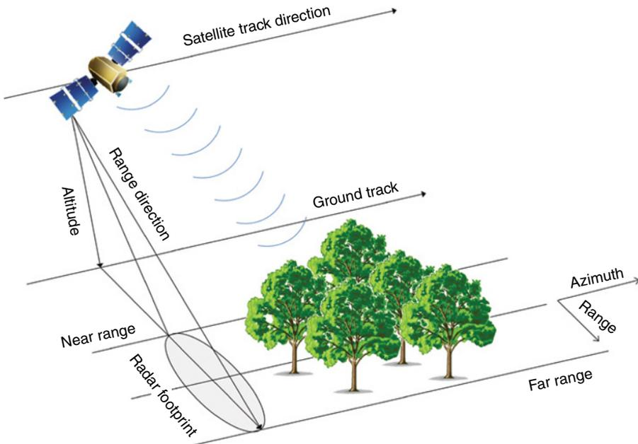
**Figure 2.1** Illustration of Synthetic Aperture Radar Satellite basic terminology.
