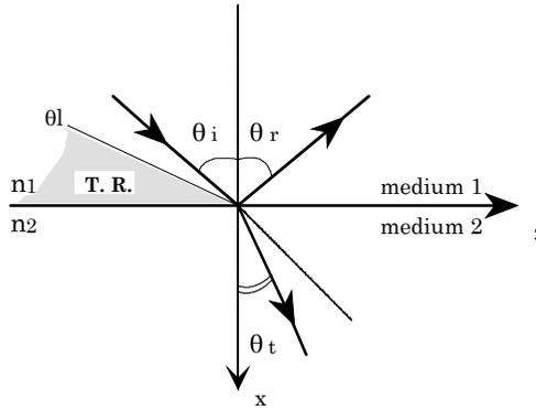
**Figure 1.2.** Reflection on an interface (medium 1/medium 2)
