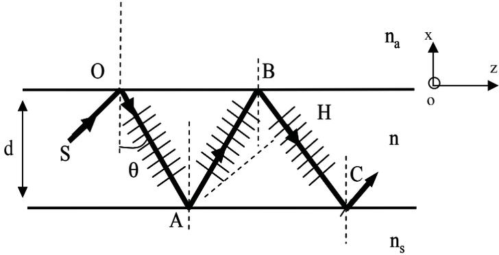
**Figure 1.8.** Propagation in zigzags within a planar waveguide
