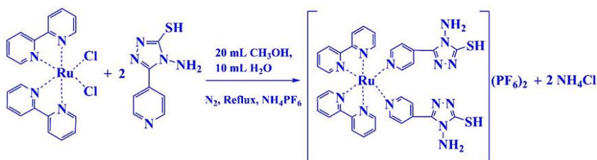
Scheme 3. Synthesis of [\text{Ru}(\text{bpy})_2(\text{apytrzSH})_2](\text{PF}_6)_2 (Complex B).
