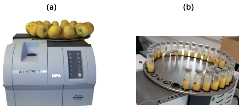
Figure 2. An example of the measurements on (a) apple and (b) purees using the NIR spectrometer.
