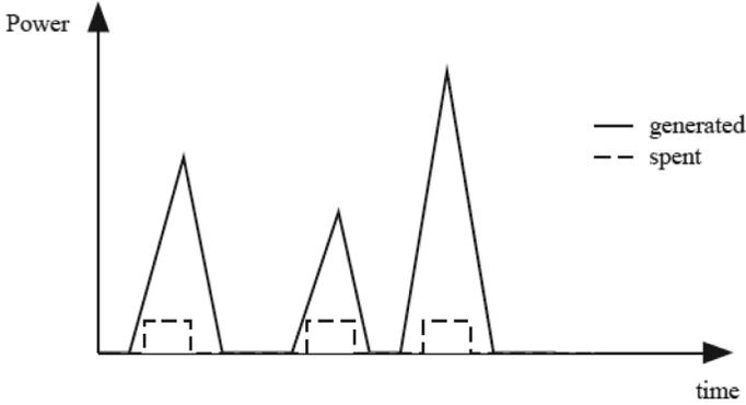
**Figure 1.5** Generated and spent power when the device operation is only at times when there is energy generation.
