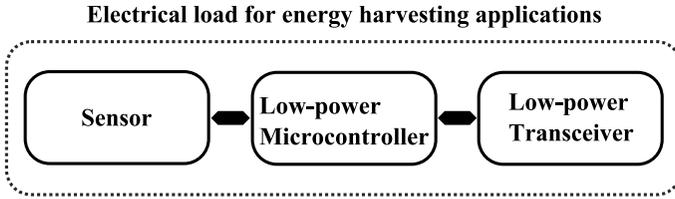
**Figure 1.3** Block diagram of a general load: sensor, microcontroller, and wireless transceiver.
