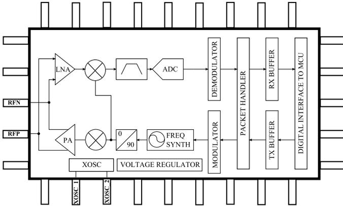
Figure 1.11 Block diagram of a low-power RF transceiver.
