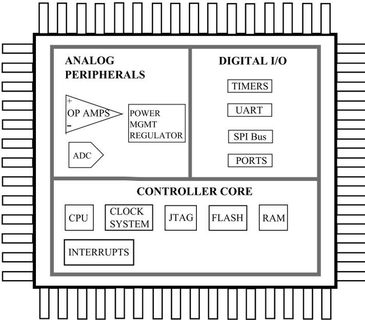
Figure 1.9 Block diagram of a low-power microcontroller.
