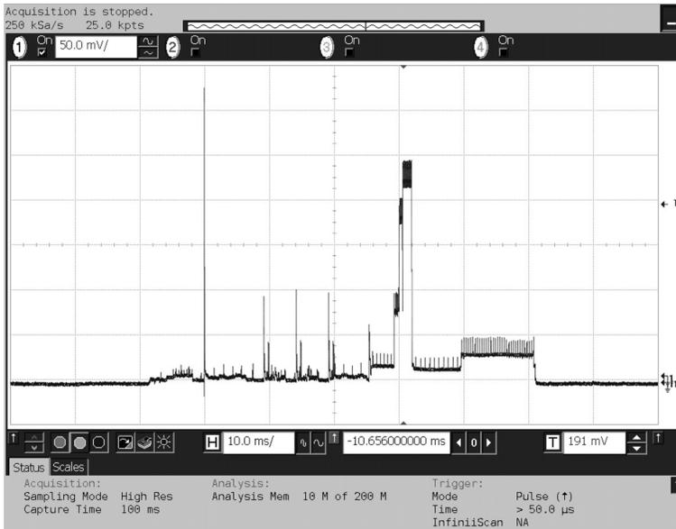
**Figure 1.7** Current profile of the eZ430-RF2500 as a transmitter in combination with an accelerometer sensor.
