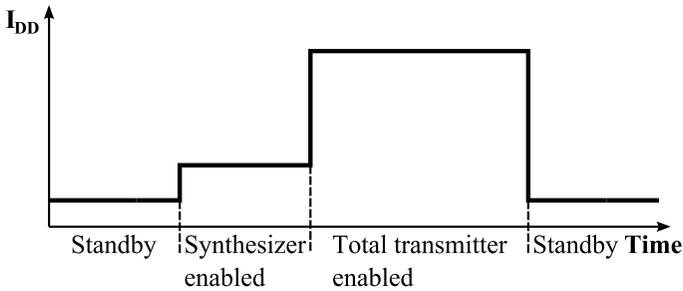
Figure 1.10 Current profile of a transceiver.
