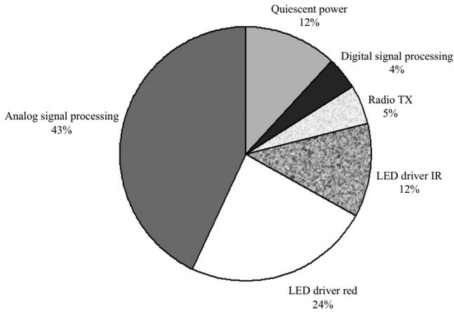
**Figure 1.8** Power consumption of the different components of the pulse oximeter device.
