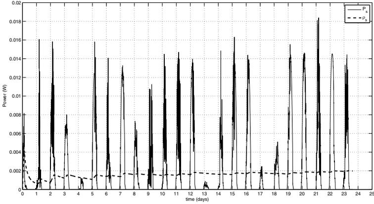
**Figure 1.12** Power  $P_s$  delivered by a portable panel to an energy storage element as a function of time and calculation of its mean power  $\rho_s$ .
