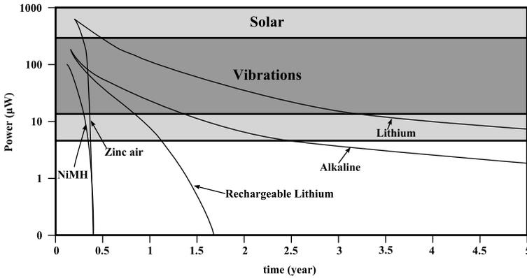
**Figure 1.2** Power density versus life time for solar cells, vibrations and batteries.
