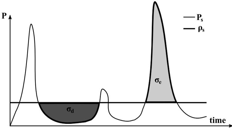
**Figure 1.13** Power delivered by the energy harvesting transducer to the energy storage element as a function of time.<sup>13</sup>
