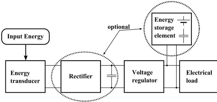
**Figure 1.1** Schema of a generic self-powered device.
