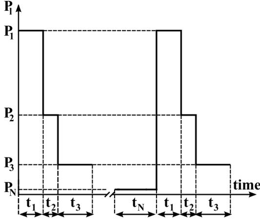
Figure 1.15 Power consumption of the load as a function of time.<sup>13</sup>
