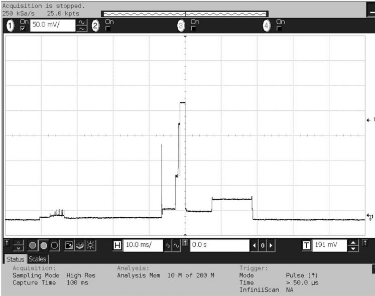
**Figure 1.6** Current profile of the eZ430-RF2500 as a transmitter.
