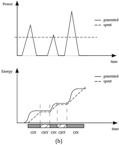
**Figure 1.4** Case of continuous (a) and discontinuous (b) load operation. In the case of discontinuous operation, the device must be turned off until enough energy is collected in the storage element.<sup>45</sup>
