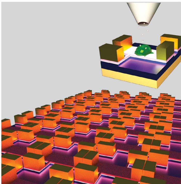
**Figure 4** Schematic representation of an AlGaIn/GaN sensor array; sensing live human cells for diagnosing diseases and developing new treatments.
