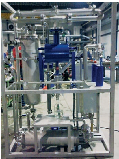
Figure 1.5: Pilot plant for recovery of ABE from fermentation using pervaporation (courtesy of Pervatech.com). The same type units may be used for bioethanol and aroma recovery
