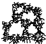
Figure 1.15 Sintered or sponge-like structure obtained by a polymerization technique separating the polymer chains.
