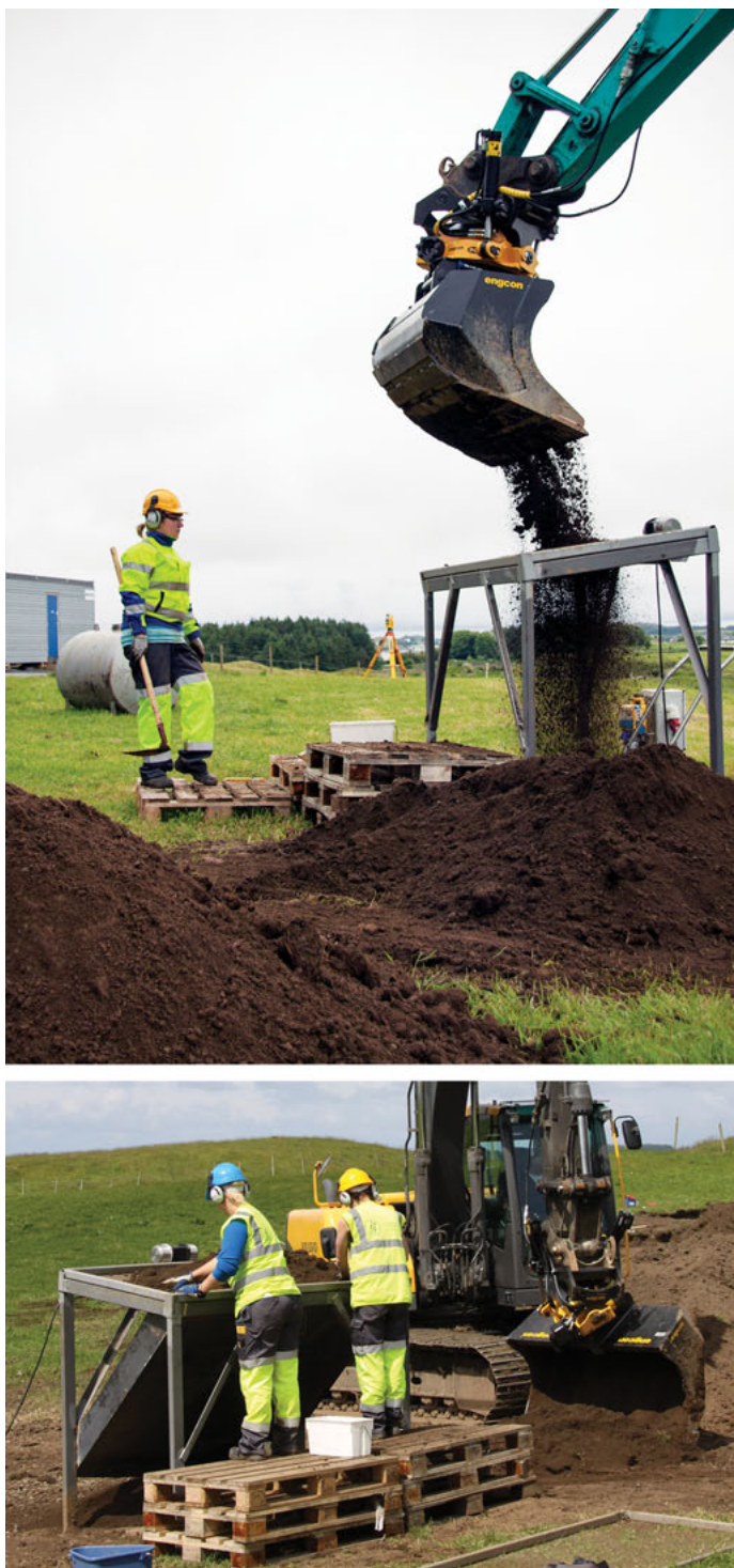
Fig. 5.4: Machine-driven sieve in use. Photo: Cathrine Glette (upper), MCH (lower).
