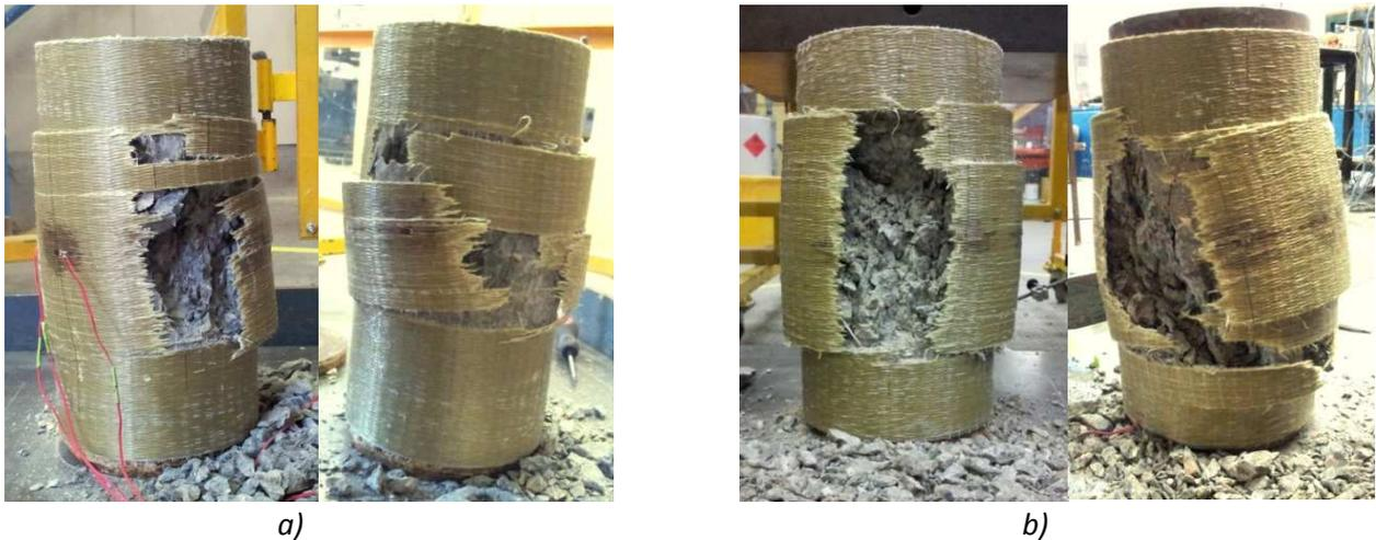
Fig. 2. Typical failure of specimens: a) NSC specimens; b) HSC specimens
