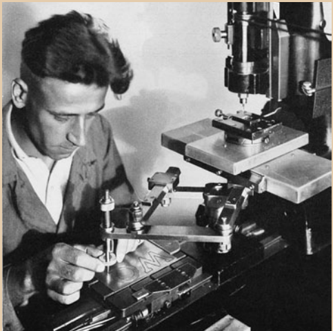
/03/ By tracing the brass template with a pantograph, the letter image is replicated as a reduced-scale matrix.
