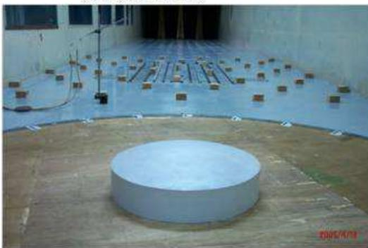
Fig.5 Testing model dome with rise-span ratio of 0.1 of B category
