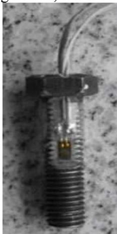
Fig.2 Bolt force sensor
