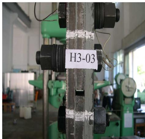
Fig.3 Mark line distortion on sample side
