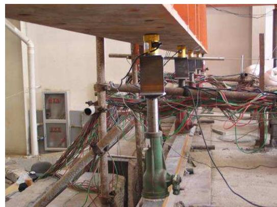
Fig. 3 View of the clamped edges
