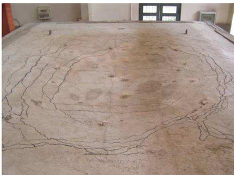
Fig. 6 Top view of the slab after fire
