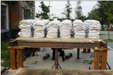
Fig. 6. Test devices of floor slabs
