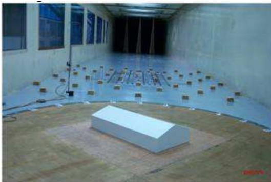
Fig.3 Testing model of B category in wind tunnel
