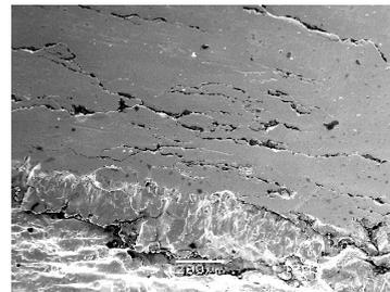
Fig. 4 Micro crack above spalling source
