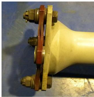
Fig.12 Example for twisting and delamination of flexible film coupling
