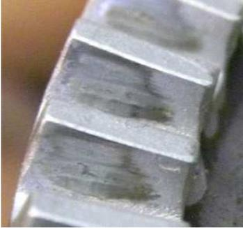
Fig. 1 Pattern and pitting area of accessory gear
