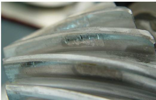
Fig.5 Scratch of a MGB collective stage pinion
