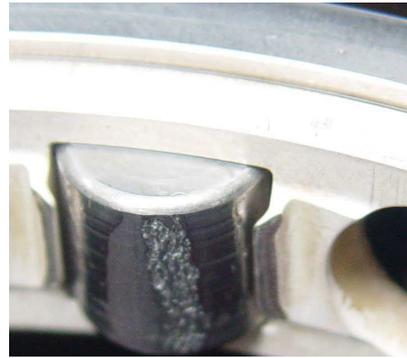
Fig. 10 Spalling of a input gear bearing roller
