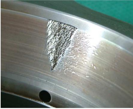
Fig. 9 Spalling of a roller bearing outer race
