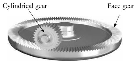
Fig.15 Face gear drive
