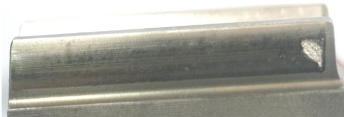
Fig. 3 Spalling of sun gear tooth
