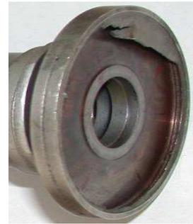
Fig.13 Diaphragm coupling breakage in the high cycle fatigue test
