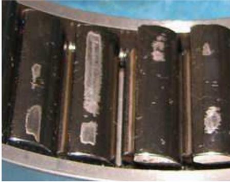
Fig. 14 Wear of sprag surface layer
