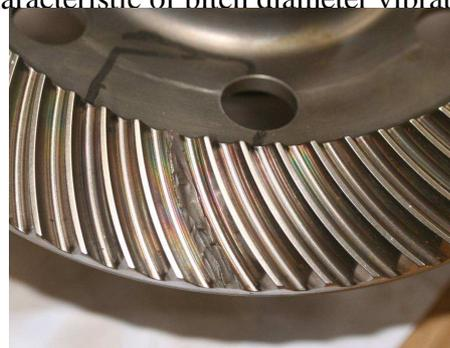
Fig.6 Breakage of gear tooth
