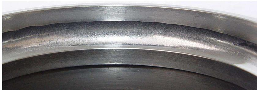
Fig.8 Spalling of angular contact ball bearing outer race (The rolling and grinding pattern is clearly near the outer side edge)
