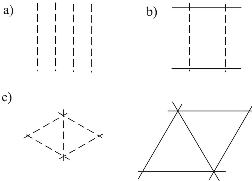
Fig. 2. Different arrays of interfacial dislocations compensating the misfit of shear type. Dashed lines represent  $\frac{1}{6}\langle 112 \rangle$  dislocations, full lines  $\frac{1}{2}\langle 110 \rangle$  dislocations.
