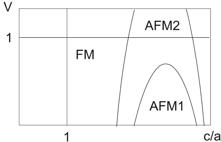
Fig. 1. Occurrence of different magnetic states at homogeneously deformed iron.  $c/a$  on the  $x$ -axis indicates the magnitude of the tetragonal deformation at given atomic volume and  $V$  on the  $y$ -axis the atomic volume normalized by the value for the bcc structure. FM, AFM1 and AFM2 are ferromagnetic, single-layer and double-layer antiferromagnetic states, respectively.
