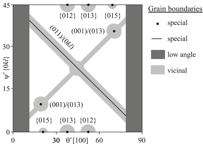
Fig. 3. Classification of  $[100]$  tilt grain boundaries in  $\alpha$ -iron.
