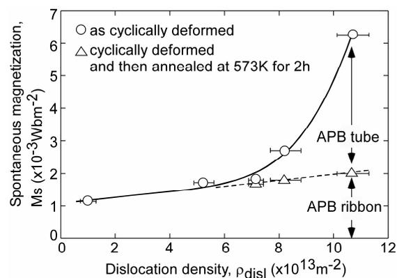
Fig.1 Variation in spontaneous magnetization of fatigued FeAl single crystals and annealed ones after fatigue as a function of dislocation density.
