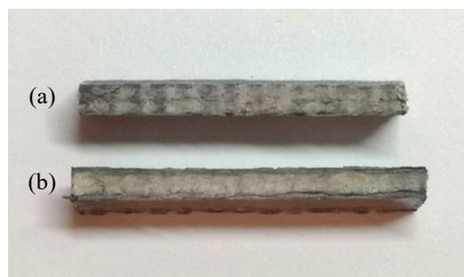
Fig. 1 Types of KCRE composite pin stacking sequence
