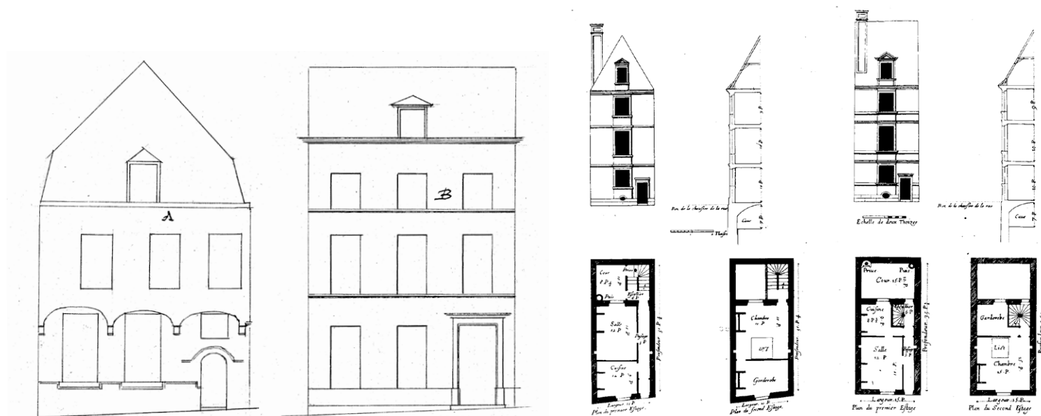
The transformation from timber (left) to brick houses (right) led to vertical window alignment and roof reversal (house transformation by Henri Partoes, Rue d'Accolay in 1819).
