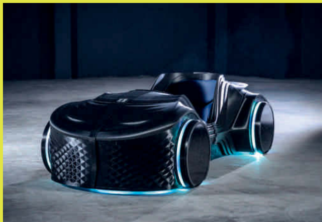
The LOCI podcar by BigRep: The fully 3D-printed, autonomous (driving) e-car
