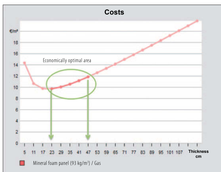
Fig. 11: Optimal cost area. The optimum is emphasised (from the minimum to 20%)
