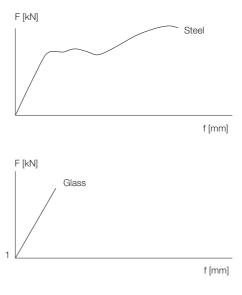
1 Comparison of the mechanical behaviour of steel and glass subjected to tension (F): whereas steel exhibits plasticity after exceeding the elastic limit and is hence highly ductile (f) up until the point of failure, glass exhibits a linear elastic behaviour up to the point of failure, without any plastic material behaviour.
