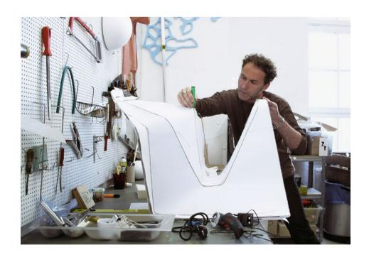
The Hemp Chair belongs to the tradition of stackable, manufactured monobloc chairs, usually made of reinforced plastics such as polypropylene. Unlike these, however, it is made exclusively from the natural fibers hemp and Malvaceae kenaf. The fibers are formed by heat treatment, and bonded using Acrodur<sup>®</sup>,
