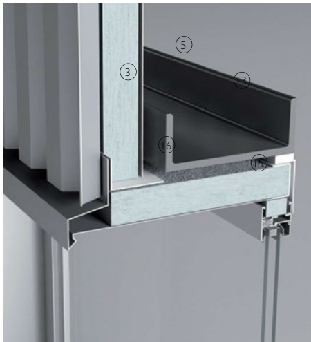
Vertical section 1:10. Aluminium window recessed into profiled metal cladding system
