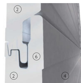
3-D views of profiled composite panel fixed to steel and of horizontal interlocking joint between profiled composite metal panels.
