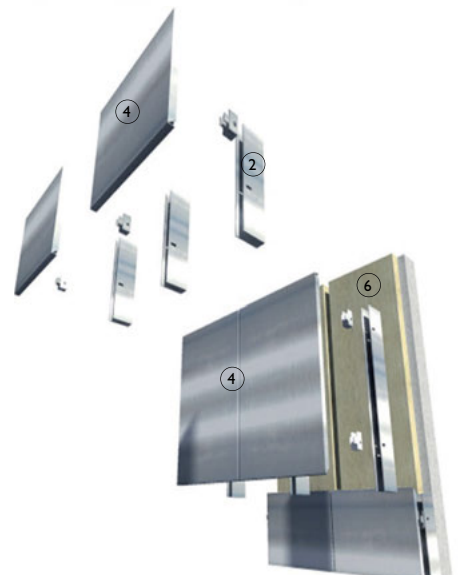
3-D exploded view of rainscreen panel system
