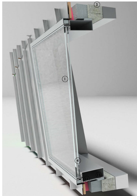
3-D view of aluminium window in folded metal cladding system
