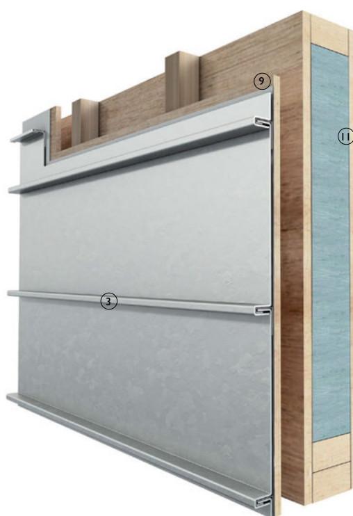
3-D view of folded metal sheet cladding with projecting joints. Type 1
