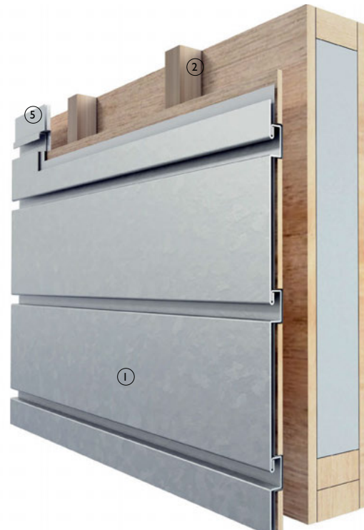
3-D view of folded metal sheet with recessed seams. Type 1
