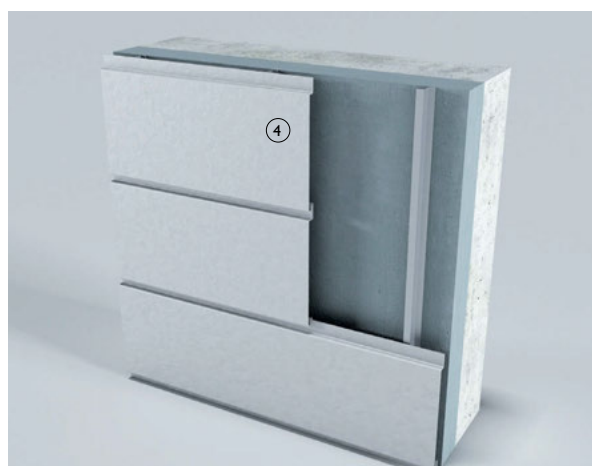
3-D views of semi interlocking rainscreen panels. Type 2
