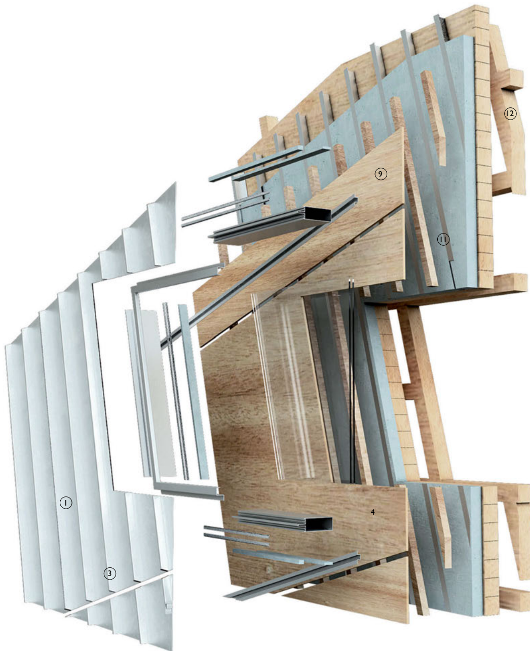
3-D exploded view of horizontally set folded metal sheet facade with angled seam lines
