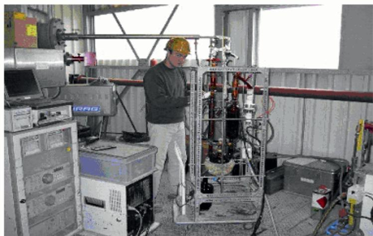
Figure 4 VDZ's emission monitoring team performing stack test as required by European and German law
