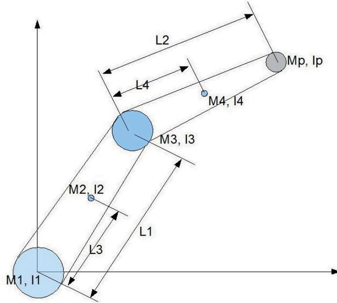
Figure 9: Two links SCARA robot
