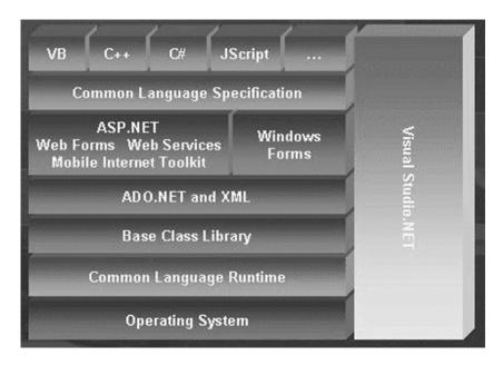
The most important component of the .NET Framework is the CLR, which provides the environment in which programs are executed. The CLR includes a virtual machine. At a high level, the CLR activates objects, performs security checks on them, store them out in memory, executes them, and garbage-collects them. The Common Type System is also part of the CLR.
