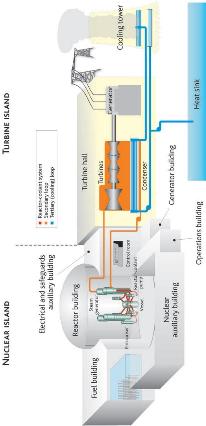
Figure 2.3. Schematic diagram of a PWR (1300 MWe or N4) and its main loops.
