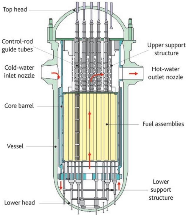
**Figure 2.5.** Cutaway of the PWR vessel at Fessenheim.
