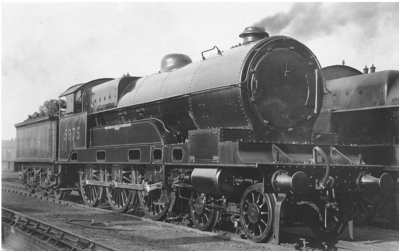
One of the twenty 'Claughtons' equipped with a larger boiler after 1928, 5975 Talisman , at Manchester Longsight depot, c1930. It was built in April 1920 and withdrawn in May 1937. (W. Potter/MLS Collection)
