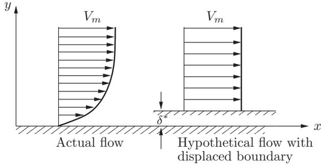
Figure 2.7: Displacement thickness
