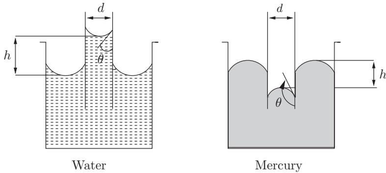
Figure 2.3: Capillary effect of water and mercury
