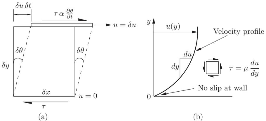
Figure 2.2: Parallel plates with fluid in between
