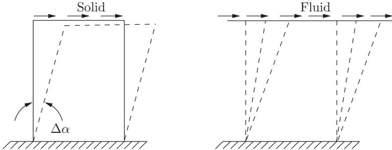
Figure 2.1: Solid and fluid elements under shear stress
