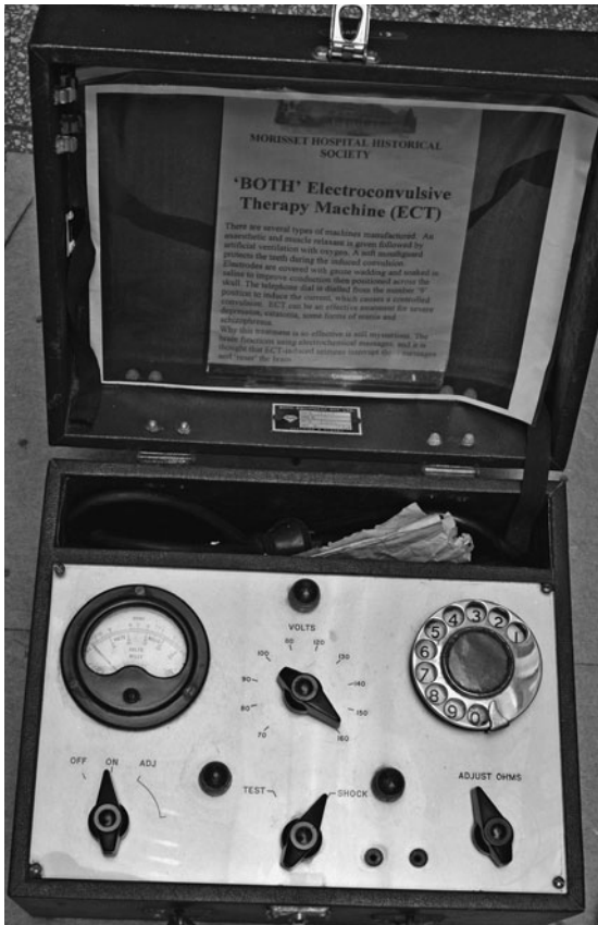
Photo 1.3.2 Dial-up ECT device with history, Morisset Hospital Historical Society, "BOTH" electroconvulsive therapy machine (ECT)
