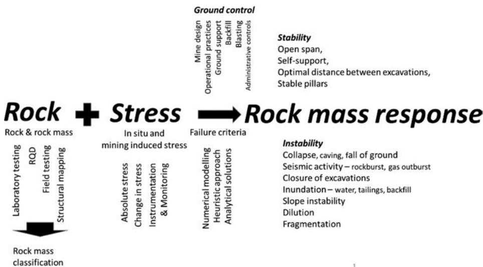
Figure 2.1 Geotechnical input to determine rock mass response.
