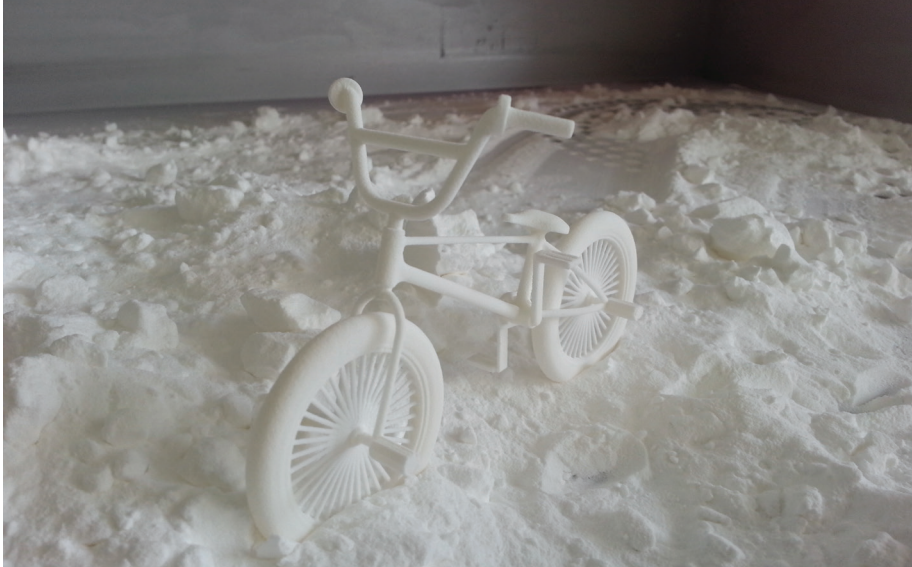
Figure 1.8 Granular Materials Binding (GMB).
