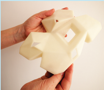
Figure 1.9b Saltygloo individually printed brick made from salt. Photo courtesy of: Emerging Objects
