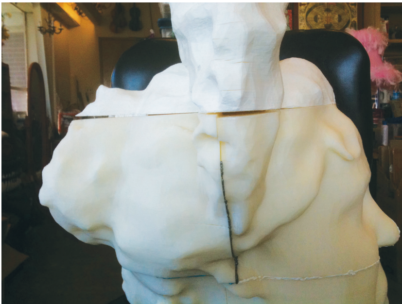
Figure 1.21 Close-up of gaps in 3D printed over-sized bust being filled by 3D printing pen. Photo courtesy of: Michael J. Horejsi
