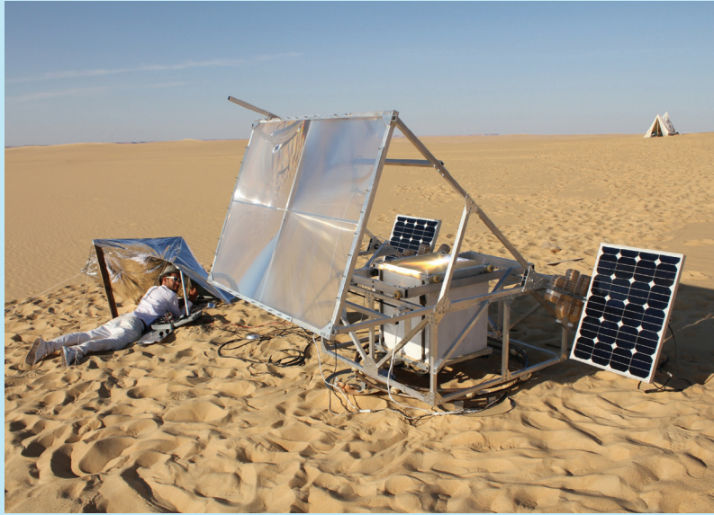
Figure 1.10 Solar Sintering printer. Photographer: Amos Field Reid. Photo courtesy of: Markus Kayser
