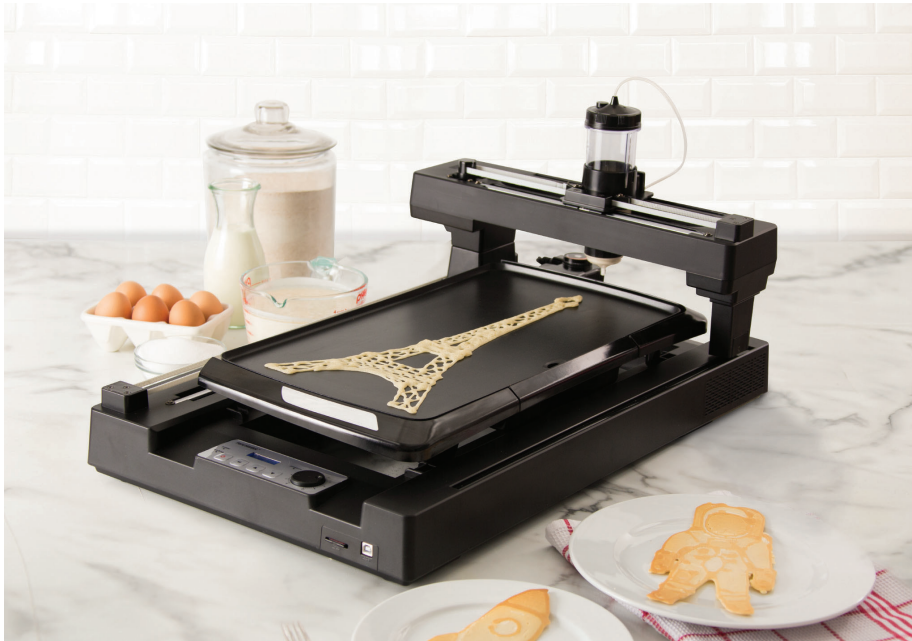
Figure 1.24 PancakeBot, invented by Miguel Valenzuela, creating a pancake in the shape of the Eiffel Tower. It uses a proprietary system to dispense the batter onto a hot griddle. Photo courtesy of: StoreBound, LLC
