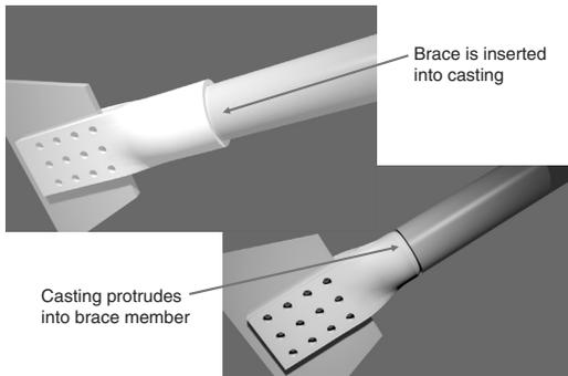
Figure 13. Cast steel connections to tubular braces for seismic load applications.
