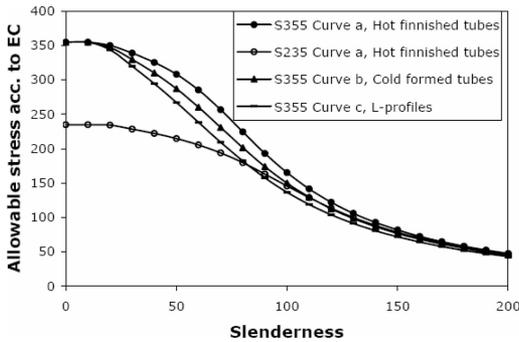
Figure 4. Buckling curves according to EC 3:Part 1-1 1992. The red curve is for tubes (hot finished) the light blue is for cold finished tubes, while the blue is for angular profiles and round bars. The green curve is hot finished tubes in steel quality S235.
