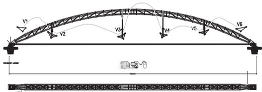
Figure 1. General cross-section of roof through the tubular steel arches.
