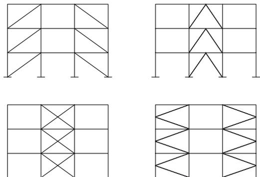
Figure 2. Typical configurations of concentrically-braced steel frames using hollow sections as bracings.
