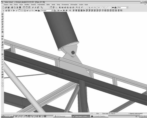
Figure 11. Detail connection for tension member x-suspension truss.
