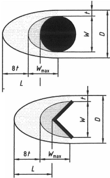
Figure 3. Ice accretion model for rime on circular and angular profiles (ISO 12492 2001).
