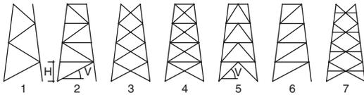
Figure 6. Typical lattice patterns (All diagonals can take compression as well as tension except pattern 4 that has special slender tension-only diagonal members).
