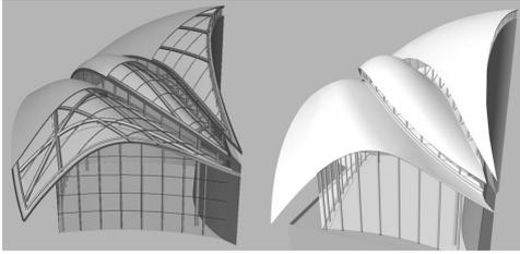
Figure 4. Two construction types: a steel structure of circular hollow sections (left) and the structural sandwich structure (right).
