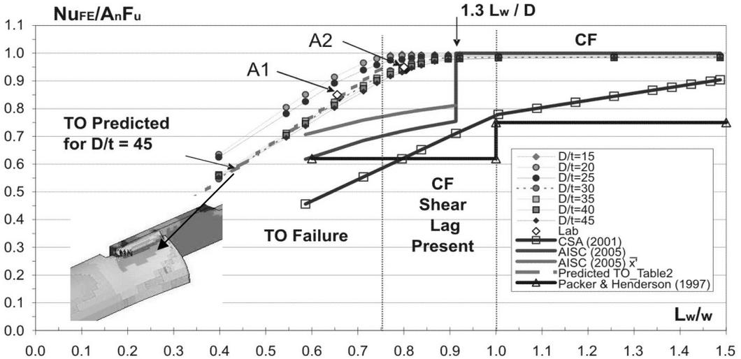
Figure 9. Results of parametric FE analysis and experiments (A1, A2) for connection type A (see Fig. 6) [Tension loading; circular HSS with the slot end not filled: a very popular bracing member detail in practice.]  $N_{uFE}$  = connection ultimate strength by FE analysis.
