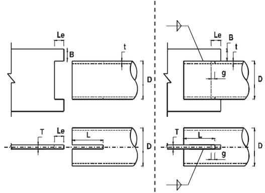
Figure 12. Fabricated connection detail using an over-slotted circular HSS but with  $A_n = A_g$  at the weld termination.
