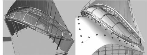
Figure 8. Two more views of the *central body*, the small cubes (image right) mark the position of the steel inserts to connect the GRP shells to the steel of the columns and the *central body* (right).
