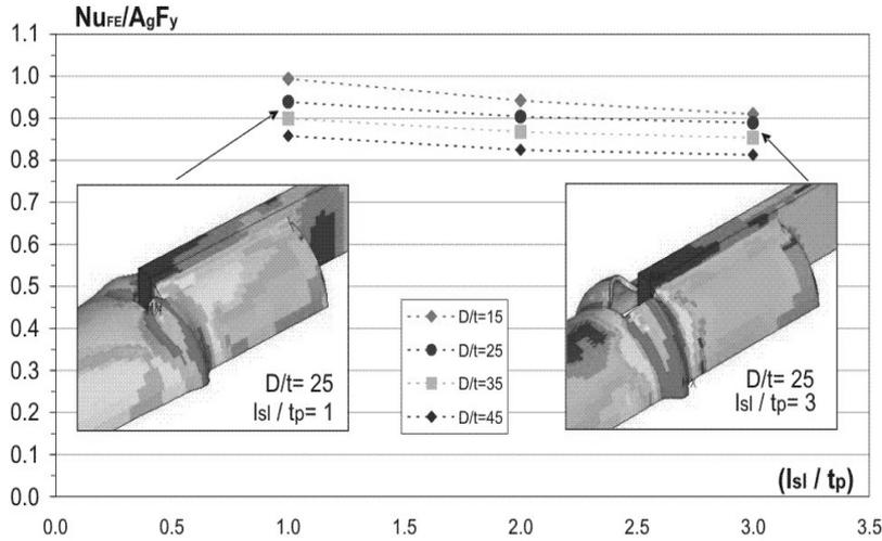
Figure 10. Results of parametric FE analysis for connection type A (see Fig. 6). [Compression loading; circular HSS with the slot end not filled: a very popular bracing member detail in practice.]  $N_{uFE}$  = connection ultimate strength by FE analysis,  $l_{sl}$  = length of open slot and  $t_p$  = plate thickness.
