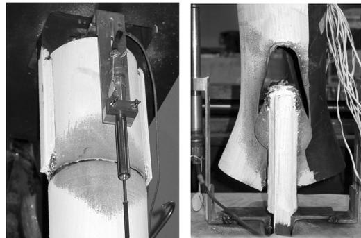
(a) Typical Circumferential Failure (CF) of the HSS, induced by Shear Lag
