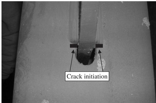
Figure 7. Example of an inserted plate with the HSS slot end roughly cut and left open.
