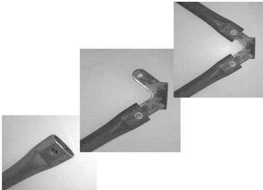
Figure 10. Principles of the assembly of the diagonals.
