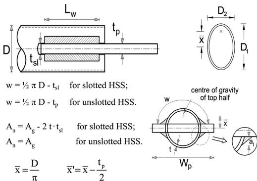
Figure 5. Important geometric parameters influencing connection design.
