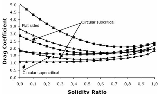
Figure 2. Drag coefficients for lattice triangular and square cross section.
