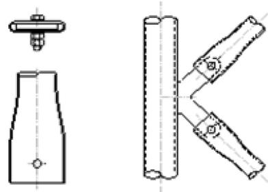
Figure 8. Special design of the joint without using welding on the diagonals.
