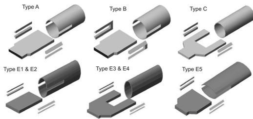
Figure 6. Fabricated connection details investigated.
