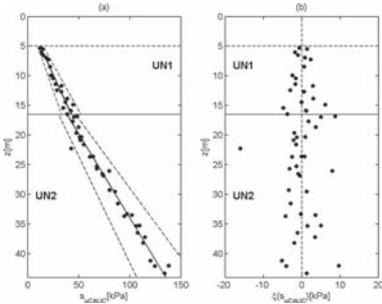
Figure 8. DSS undrained shear strength: (a) trends and standard deviations; (b) residuals of detrending (Uzielli et al. 2006a).
