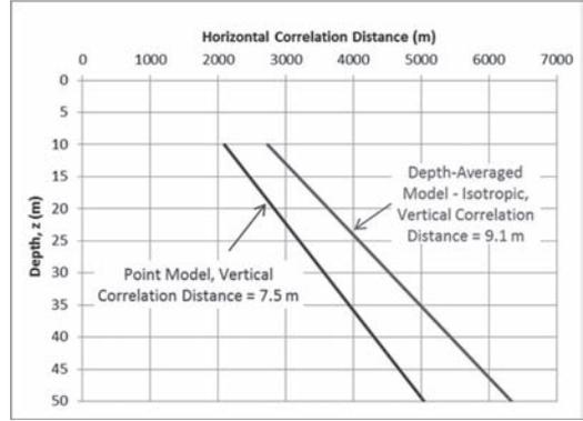
Figure 2. Horizontal correlation distance<sup>2</sup> versus depth for point and depth-averaged values of design undrained shear strength in random field model (from Cheon & Gilbert 2013).
