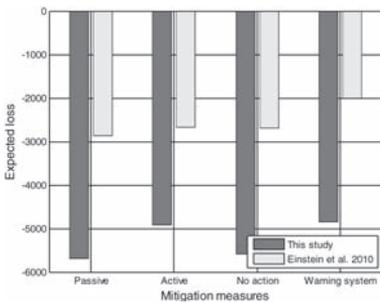
Figure 18. Losses for ‘no action’, ‘active measures’, ‘passive measures’ and ‘warning system’ (after Nadim & Liu 2013a).
