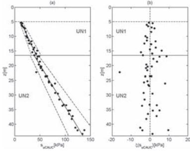
Figure 7. CAUC undrained shear strength: (a) trends and standard deviations; (b) residuals of detrending (Uzielli et al. 2006a).
