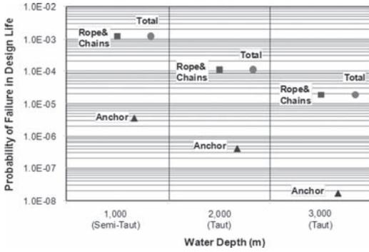
Figure 17. Comparison of probabilities of failure in design life for different components in the most heavily loaded line of a mooring system (from Clukey et al., 2013).
