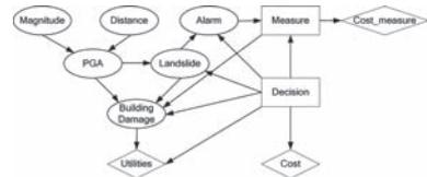
Figure 14. Decision making Bayesian network for earthquake-triggered landslide risk assessment (after Einstein et al. 2010).
