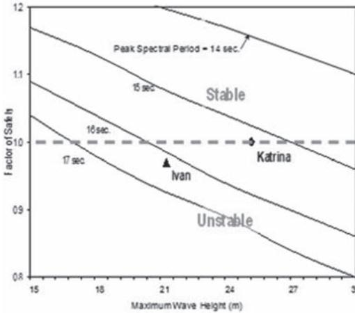
Figure 12. Factor of safety for slope failure versus wave height and period at one location in Mississippi River Delta (from Gilbert et al., 2010).
