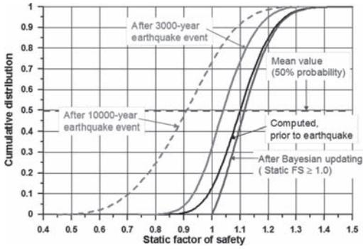
Figure 11. Results of probabilistic analyses of static undrained stability, prior to (black), updated (blue) and after the 3,000-year and 10,000-year earthquake event (red) (from Nadim 2011).
