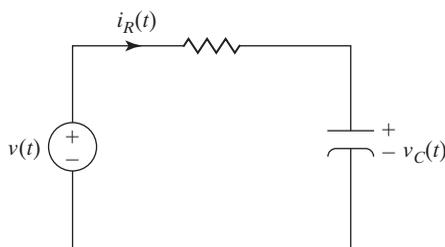
**Figure 1.1** Resistor-capacitor circuit.
